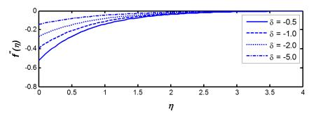
Fig. 1. Dimensionless velocity and shear stress profiles at s=1 and  $\gamma=0.5$  for different second-order slip parameters.
