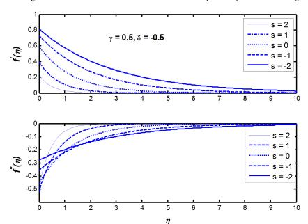
Fig. 3. Dimensionless velocity and shear stress profiles at  $\delta = -0.5$  and  $\gamma = 0.5$  for different mass suction parameters.
