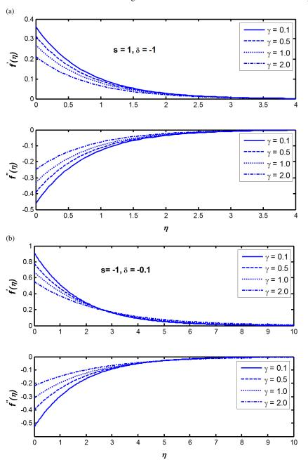
Fig. 2. Dimensionless velocity and shear stress profiles at  $\delta = -1$  and s = 1 (a) and  $\delta = -0.1$  and s = -1 (b) for different first-order slip parameters.
